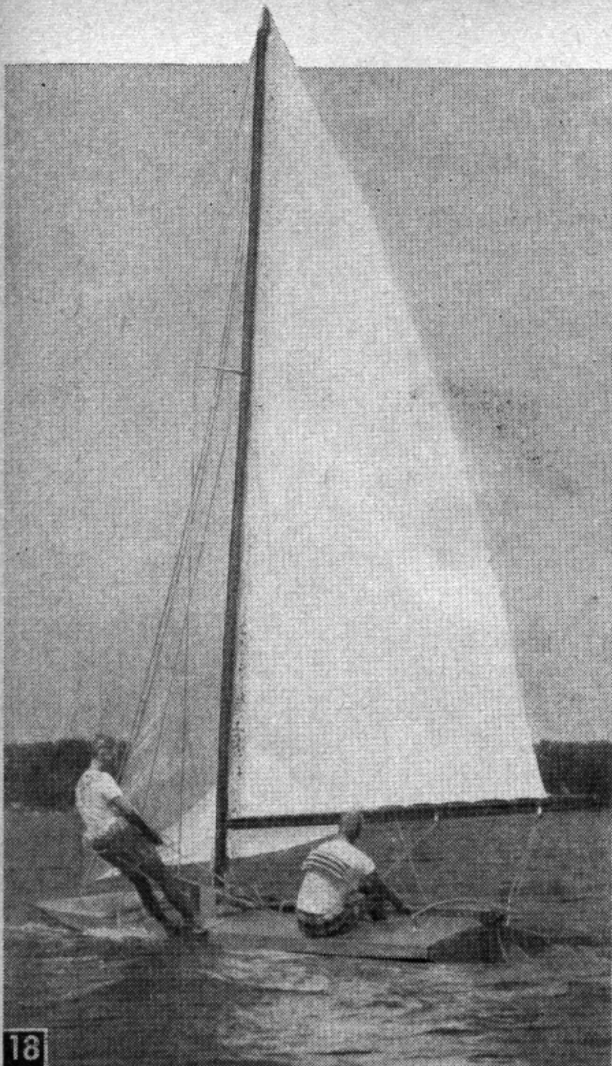
One crew member out on the hiking board can exert as much weight to balance sail pressure as two crew members leaning out over the hull sides without hiking boards. Board can be quickly moved from side to side.
