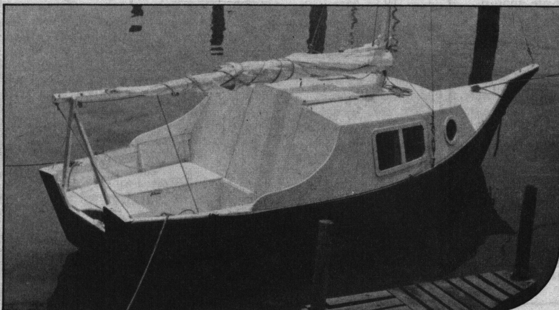
Completed boat showing cockpit, sliding hatch and the companionway door.
