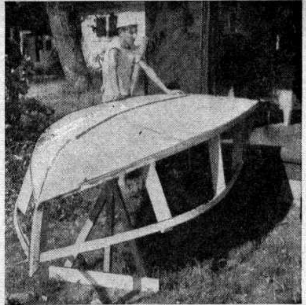
The short piece of plywood at the stem should be softened with hot water so as to bend readily into its final position.
