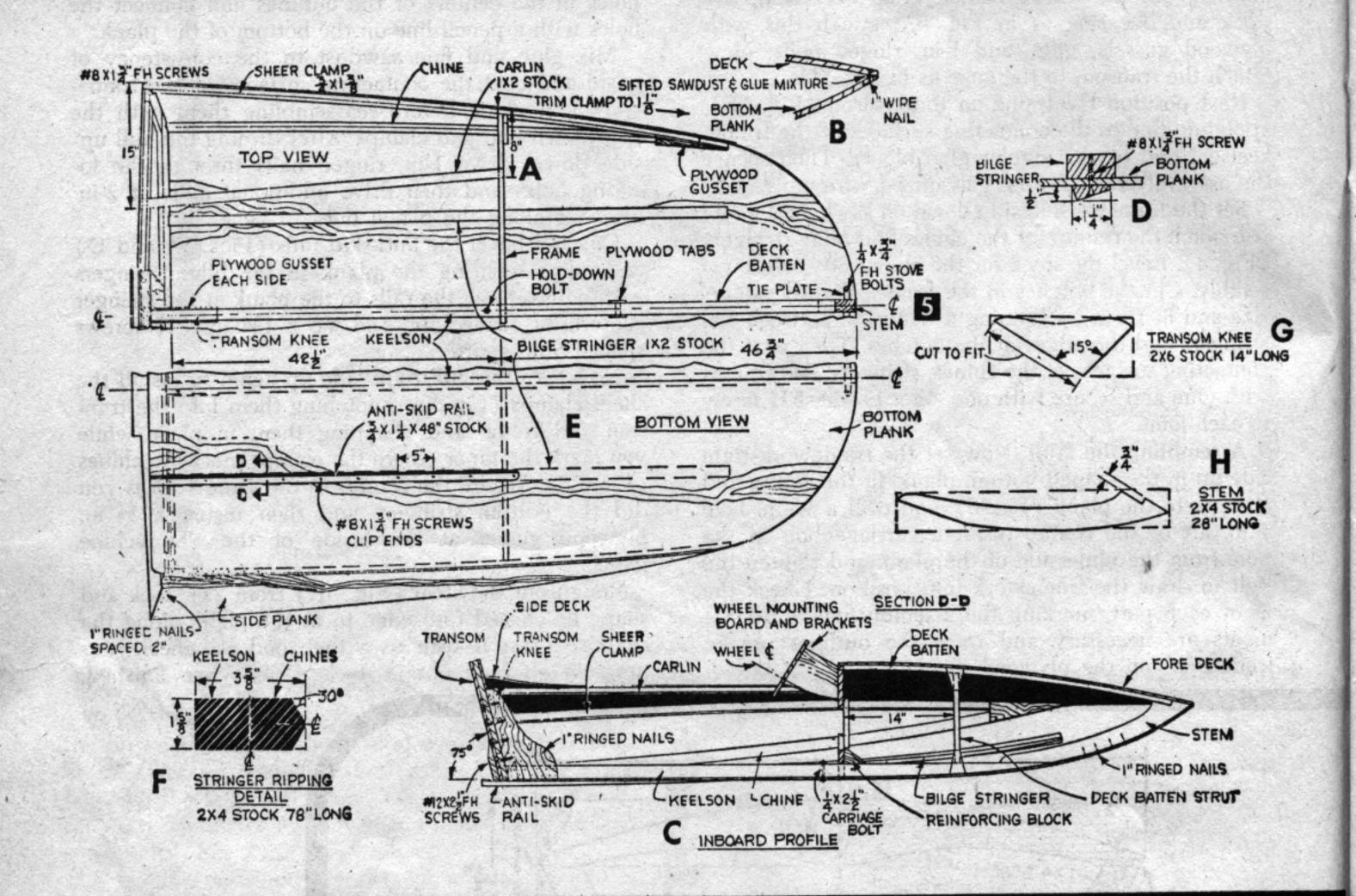
coat the stem, keelson, and plank with glue and install the stem with 1-in. ringed nails driven at 1½-in. intervals through the plywood on each side of the slit.
