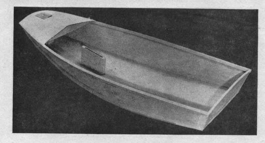
Caulk all interior joints and seams before turning the hull to complete the underside. Coat contacting surfaces of the mast step and daggerboard and case with putty for a waterproof joint.
