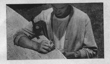
3: Use simple overhand stitch. Use Nylon lacing, start with three holes at each end of seam, tie off. Begin again at middle, work toward ends.
