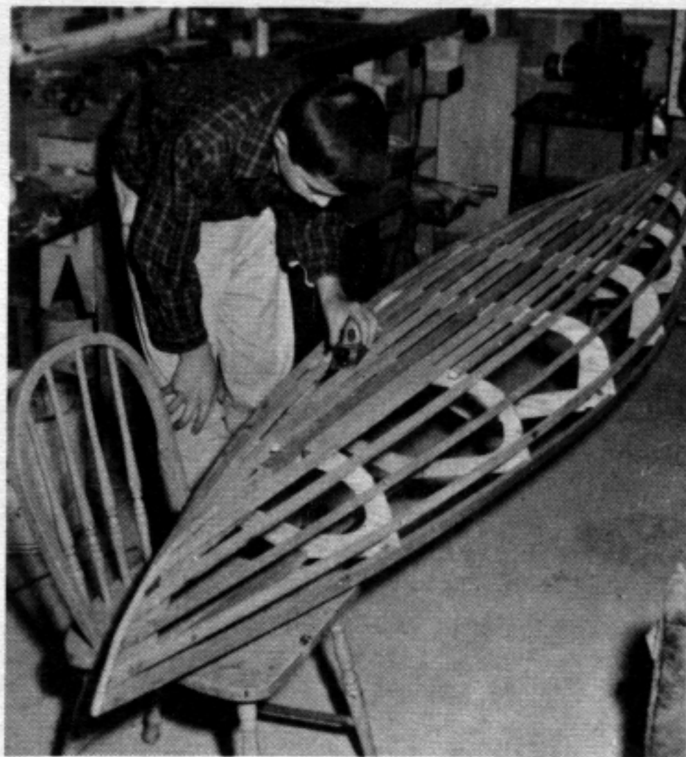
All edges of the completed boat frame must be planed and sanded smooth so that the canvas cover will not wear at any spots. This is important.
