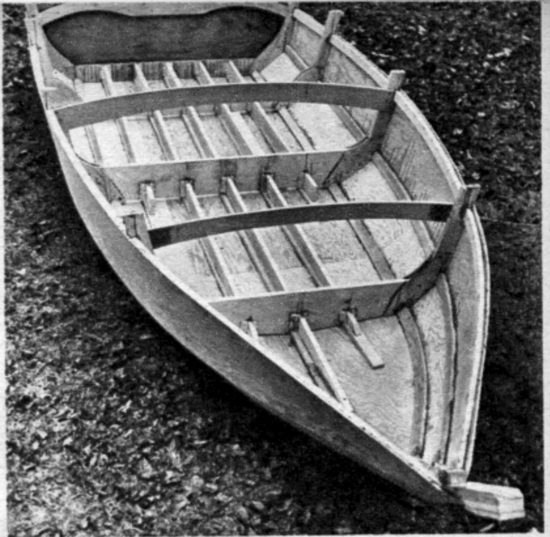
The boat is now completely planked and turned right side up, ready for the finishing touches.
